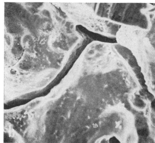
Figure 2 Scanning electron micrograph of the as-cast Al-3.7% Cu-0.11% Ti alloy, corroded for 12 days. (a) × 200, (b) × 500.
